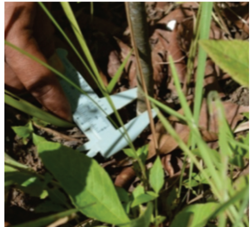
Figure 28. Root collar diameter of newly planted seedlings are monitored using a vernier caliper.
