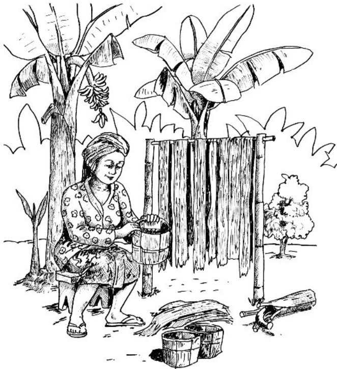
Location for drying flattened banana trunk material on a rack
