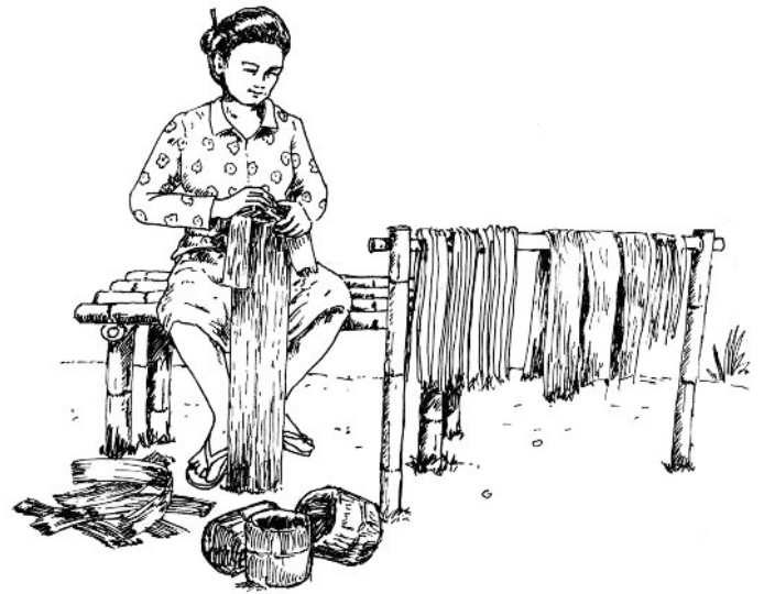
Set up of the location for production of banana fiber pots of different sizes: Posts with different diameters (10cm-30 cm) are placed in a way that a person sitting on the bench can work comfortably at each post and reach at the same time the banana fiber materials U flattened and dried trunk material and dried banana fiber strings.
